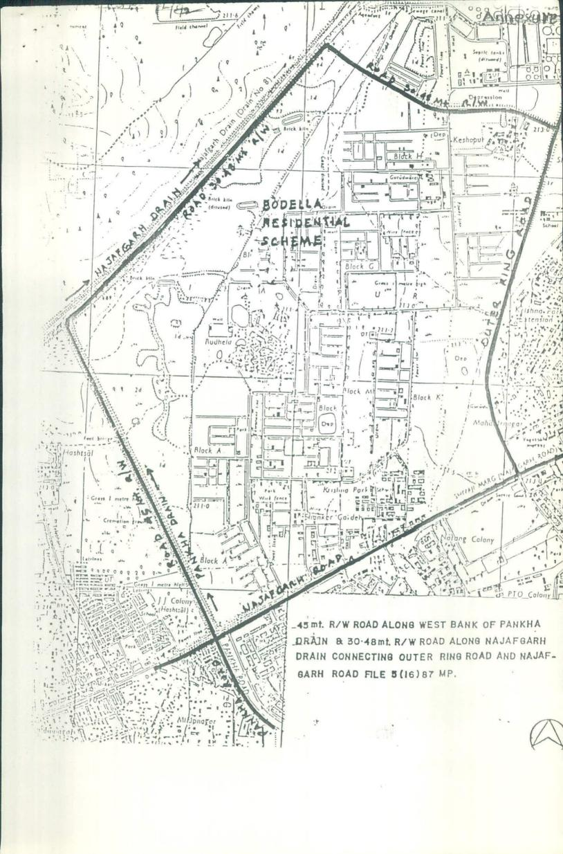
Sub: Composite alignment plan of 45 mtrs. M/W road along west bank of Pankha Drain & 30.48 mtrs. R/W road on the eastern side of Najafgarh Drain connecting outer ring road and Najafgarh Road.
